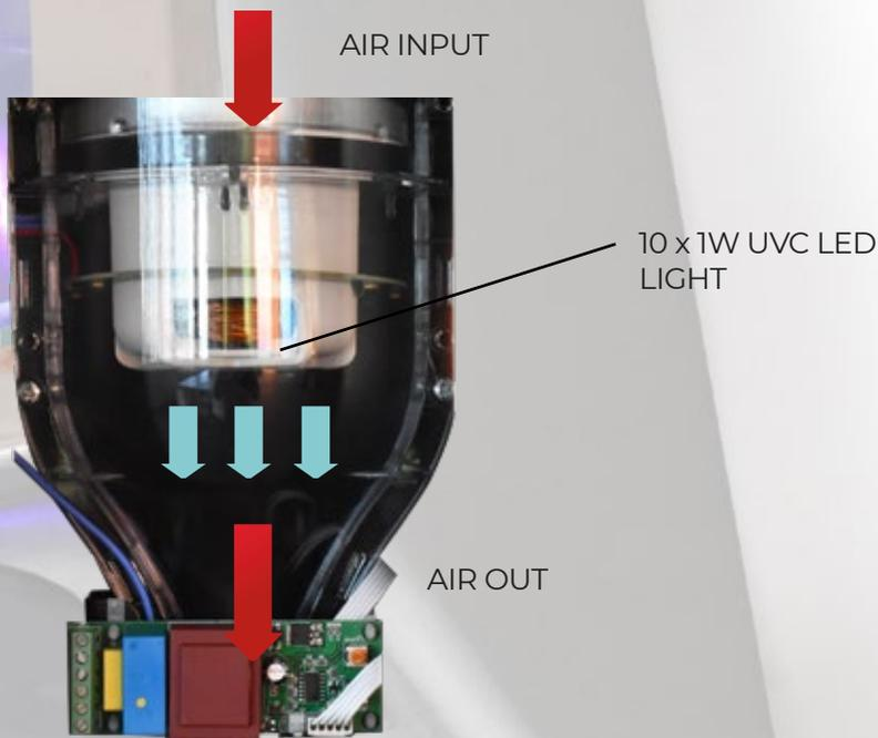
UVC led module irradiate instantly all air flow without delay can be produced in fluorescent tubes.
